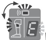
**When I turn on the Control Unit, it beeps, the Control Unit and RF Stim Unit indicators alternately flash RED, and "E" flashes in the digital display. The RF Stim Unit indicators are not lit.**
