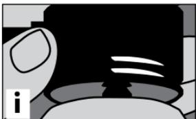
**i** Install pin on liner. Engage lock to check for play between lock and liner.
