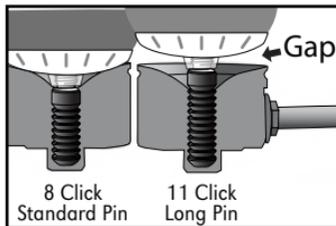
**G1** Do NOT use 11 click long pin on unconverted standard Air-Lock, the long pin will bottom out and create a gap between lock & Liner.
