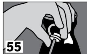
Expose fabrication plug and remove.
