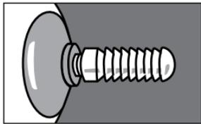
**H4** If a Gap is created between the pin and liner.
