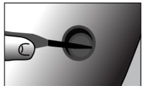
**S13** If the inside of the lock is crusty take a pick and loosen it up and remove the dirt.
