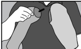
**S18** Do an engagement test with the pin and liner into the lock to make sure everything is working to your satisfaction. 5 to 6 clicks and you cannot pull pin loose.
