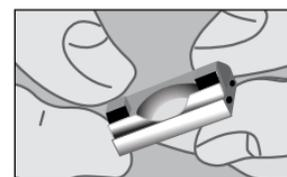
**S7** White marring, worn down tooth and worn O-rings are good indicator the internal parts need replaced.
