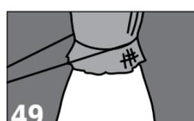
Tie second layer of composite under five hole plate and reflect down over mold.
