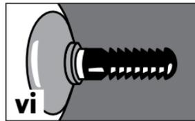
**vi** Replace pin on adaptor, making sure base fits snugly on pin spacers.
