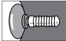
**H6** Replace pin on adaptor, making sure base fits snugly on pin spacers.
