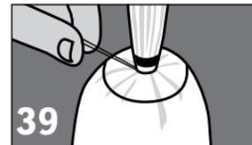
**39** Pull inner PVA bag over mold. Bag may be heated to help conform to distal end. Tie PVA to anchor in the tie-off ring.
