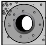
If you are having trouble engaging the pin and the lock funnel is scratched and pock marked from the pin this could be a sign of poor pin alignment which can be caused by not aligning the liner and pin correctly or the lock is not aligned correctly in the socket.
