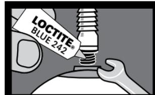
**H8** Apply Loctite® Blue 242 to threads of lock pin. Pin may need to be tightened with a 7/16" or 11 mm wrench. (See Caution #5)
