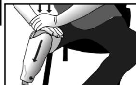
**P2** Performing a CPR motion on the knee can help the pin engage with the lock plate. Get at least two clicks before standing.
