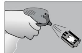
**S9** Clean off parts with rag and rubbing alcohol or acetone.
