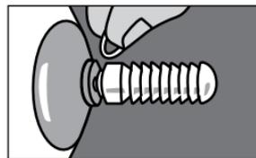
**H5** Based on the size of the gap created by loosening pin, install appropriate number of pin spacers on threaded end (see Caution #5).
