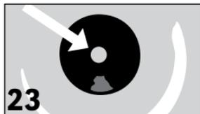
**23** Place lock pin in lock to hold lock plate.
