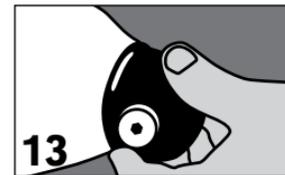
**13** Place lock on mold. Mark desired location of release button. (See Caution #1)
