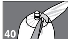
**40** Trim excess PVA material between tie-off groove and O-ring. Keep O-rings clear.
