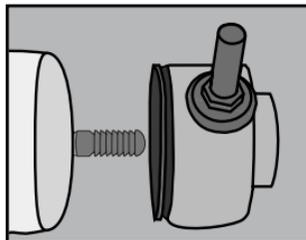
Order a fitting lock from Coyote to help with pin spacer adjustment. The reinforce distal end of the fitting lock helps give a more accurate reading on how many pin spacers to use.
