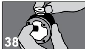
**38** Remove all lock parts before laminating. Put wax or clean clay in fabrication plug hole.
