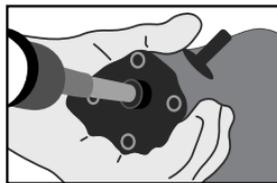
**G4** Using 5/8" Hole saw and 5/8" countersink enlarge the drill hole to accept the Pin Cap.
