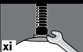
**xi** Now tighten pin assembly with 7/16", 11 mm wrench or vice grips to insure complete thread engagement of brass into liner and pin into brass. (See Caution #4, #5, #12)
