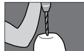
**7** Drill 1/2" diameter hole. Angle hole to help anchor adhesive.
