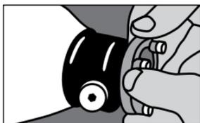
**16** Place the provided adhesive foam on the four connector posts. Place connector offset or centered.
