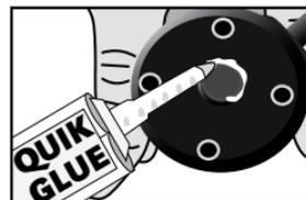
**G8** Use Coyote Quik Glue or 5 minute epoxy and glue around edge of Pin Cap. Let glue set and remove guide pin.
