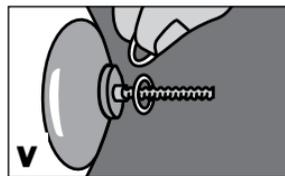
**v** Based on the gap size created by loosening pin, install appropriate number of pin spacers on the adaptor (see Caution #5).
