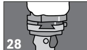
**28** Use Coyote alignment coupler CD106 for alignment during fitting.
