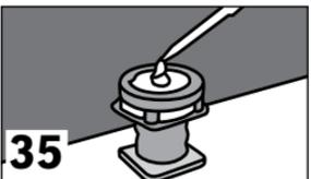
**35** Separate lock from connector. Fill connector with Coyote Quik Glue or fast-setting epoxy.
