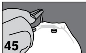
Ensure the four post holes of the connector are exposed. A hot nail or awl can be used.
