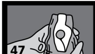
Reinforce with carbon tape between posts. Avoid extra material around fabrication plug for easier removal.
