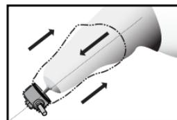
Make sure the pin slides straight into center hole in socket lock. Clicks should be one at a time.
