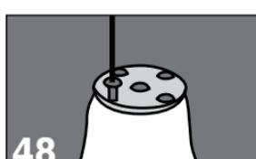
Lubricate screws and install five hole plate. (See Caution #C4)
