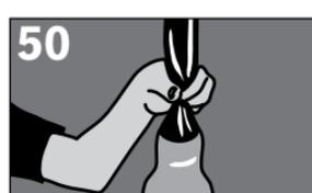
Pull bag and laminate as usual. Initially restrict flow to center hole on plate, forcing out air pockets.
