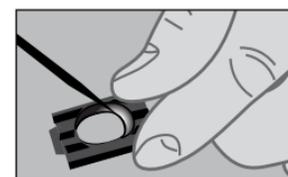
**S8** Check lock plates tapered sloped edge and the teeth on the pin for excessive wear.
