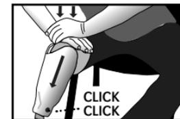
Performing a "CPR" motion on the knee can help the pin engage with the lock plate.
