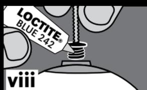
**viii** Apply Loctite® Blue 242 to threads of lock pin on adaptor screw 10 mm threads. Screw into liner finger tight.
