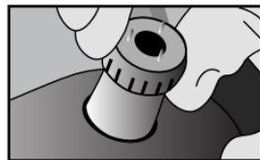
**S5** Use lock wrench to remove valve body (recommended) or 13mm deep well socket.
