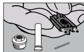
**S6** Take lock apart and inspect internal parts for wear, bad O-rings and bent or rusted springs.
