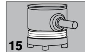
**15** If using the Deep Air-Lock add the three Spacer Disks to the lock before adding the connector.
