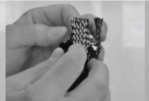
7. Fold carbon and other layup materials between connector posts. As layup material is added, ensure the connector posts remain exposed.
