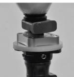
4. Lower mold and lock onto connector. Allow glue to set.
