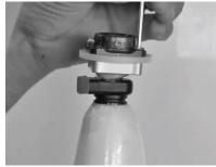
5. Remove screws from connector.
