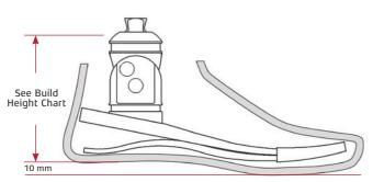
Note: Build height measurements represent a fully assembled unit.
